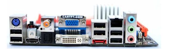
The Zotac mainboard convinces by the high number of possible ports. The well equipped I/O panel offers the following possible ports: 1x VGA (DSUB-15), 1x DVI, 1x HDMI, 6x USB 2.0, 1x eSATA, Audio, 1x LAN 10/100/1000 MBit, SPDIF (optical + coaxial), WLAN antenna, 1x PS/2 (Keyboard).
