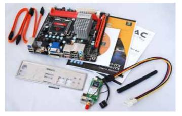
The appeal of the debut feature of Zotac on first sight is the high performance onboard graphic which will be enjoyed by the HTPC, CarPC user as well as the gaming enthusiasts. Furthermore, the Zotac mainboard scores thanks to a high degree of connectivity. For example, it provides 12 USB 2.0 (6x internal, 6x external) ports, VGA, DVI, HDMI and a WLAN modul which is part of the delivery content.
