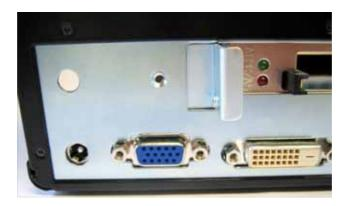
6. Screw the angle bracket from the outside on to the I/O panel.
