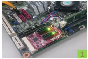
Please connect EMPS-32R1 to onboard mPCIe slot.
