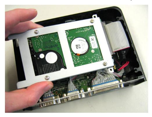
Install the HDD mounting unit into the enclosure again:
