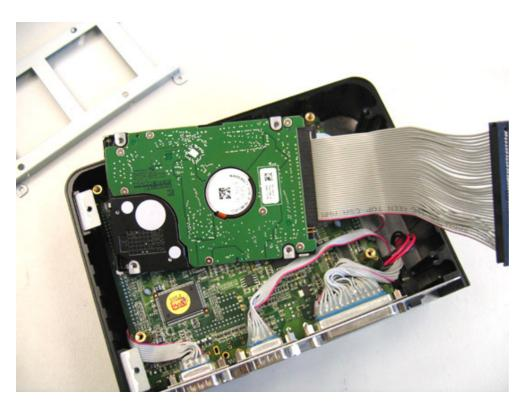
The 4 screws of the HDD are needed to install the HDD onto the mounting unit:
