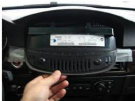
STEP 4: Pulling downwards and slightly angling the unit will allow the unit room to come out of dash.
