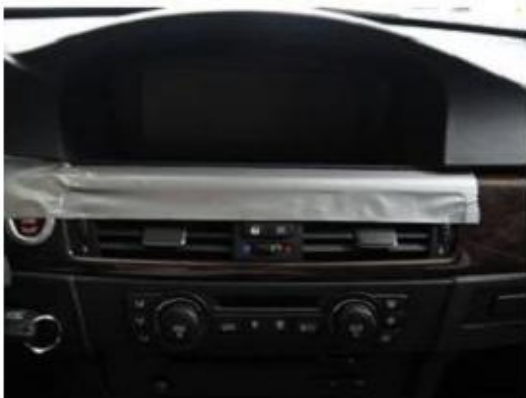
STEP 1: Protect dashboard first by laying tape on dashboard trim.
