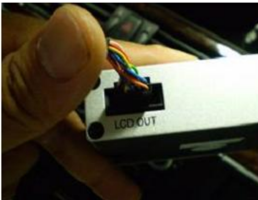
STEP 7: Connect supplied LVDS Cable To LCD OUT side of the INTERFACE
